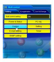
The multi controllable menus are "Power & Status", "PC adjustment", "Control", "Setting", "E-mail setting", "Timer", and "SNMP setting". Click each menu and perform setting and adjustment.
